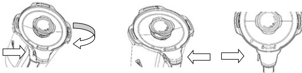
Put the jar onto the main body at the correct direction and sit properly, or else the motor cannot be started.
